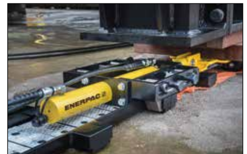
▼ Low-Height Skidding System assembly (LH400).
